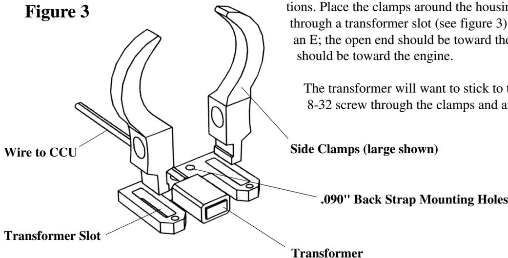
The transformer will want to stick to the magnets; that's OK. Put the 8-32 screw through the clamps and attach the 8-32 lock nut. Tighten the nut enough to remove most of the play from the clamps -- you will have to move things slightly for final adjustment.
